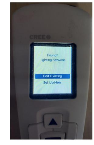
2. Turn on the Configuration Tool and connect to your SmartCast network.
